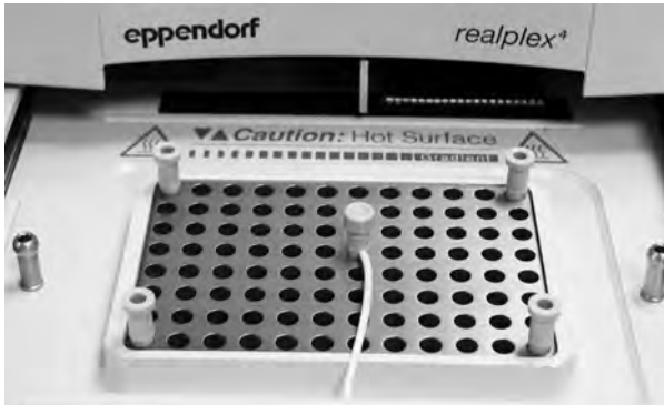
Figure 3: Spacers in thermoblock of Mastercycler ep realplex
