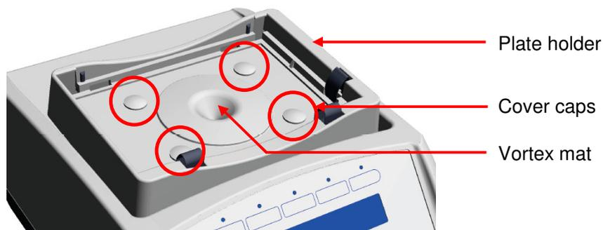
Vortex mats starting with S/N 10001 are glued to the plate holder to prevent liquid from entering the device. That meant that the vortex mat could no longer be removed and the screws below it, which are used to disassemble the device, could not be removed. Repair or service of the MixMate was temporarily unavailable.
